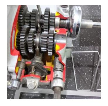
4 speed positive stop gear box internals
