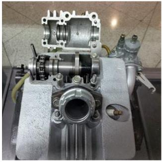
2 stroke with 4 stroke exhaust valve gear
