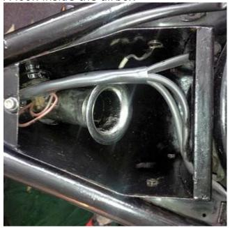
Contacted carb supplier Adam Jahn who supplied 2 smaller diameter 0.93 and 0.82 mm needle jets. For first time ever the plug came out with no soot, still black on the outer electrode but deep brown on the centre electrode. Also the bike pulled as I had expected a 4 stroke single to do. The carb needle is at its lowest, weakest mixture notch, so a careful eye will be kept on carb colour in case it suddenly chalks up and risks the valves.
