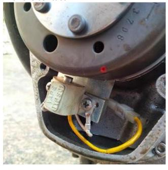
Timing with points fitted requires the crankshaft marker stamp of ZP Zundepunkt , ignition point, to be visible through the peep hole under a rubber bung in the crankcase wall which is 10 degrees before top dead centre.
