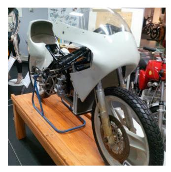
80cc 2 stroke disc valve racer
