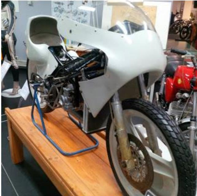
80cc 2 stroke disc valve racer
