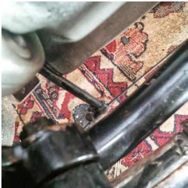
Actuating lever fouling the gearbox housing
